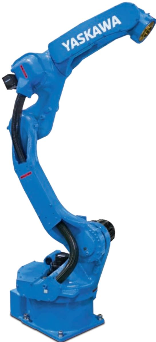
The MOTOMAN GP12 is a fast and precise 6-axis industrial robot with a payload capacity of up to 12 kg. With a reach of 1440 mm and a high repeatability of  $\pm 0.08$  mm, it is ideally suited to assembly tasks, but also universal handling tasks, CNC machine tool tending or packaging. Its streamlined modern industrial design minimizes the space requirements at the installation site.
