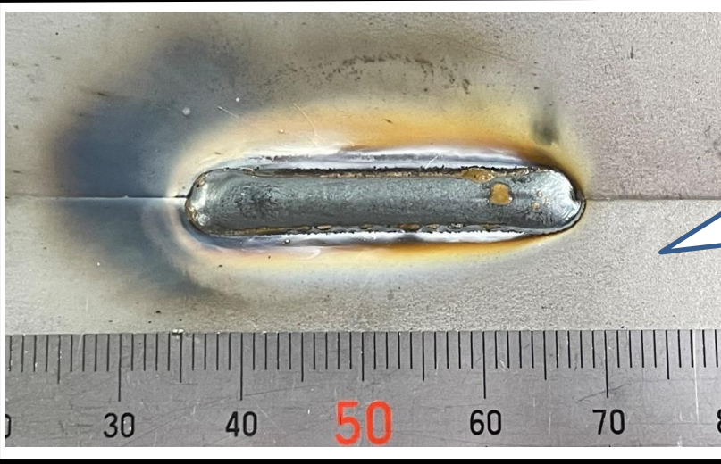
Push-arc process 85 A, 16 V, 80 cm/min. Galvanized sheet steel, thickness 1.0 mm Butt joint (wire diameter \phi 1.0 )
