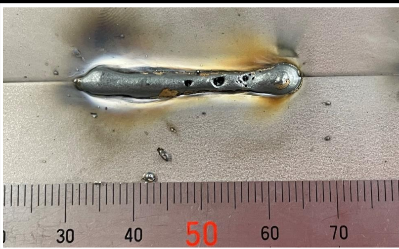
Conventional Synchro-feed 85 A, 16 V, 80 cm/min. Galvanized sheet steel, thickness 1.0 mm Butt joint (wire diameter \phi 1.0 )
