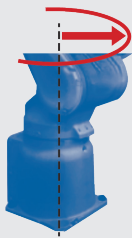
Former model MH5(L)S II Interference radius: 182 mm
