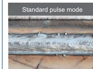
Spatter adhesion and undercut occur
