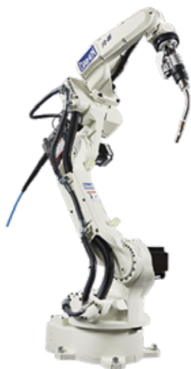
FD-V8 8kg payload, 1400mm reach
