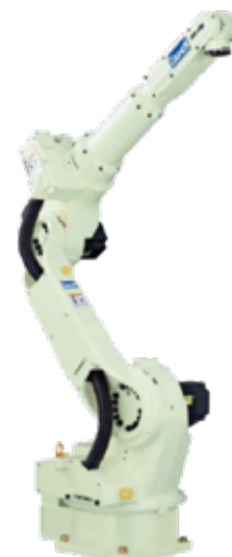
FD-V8L 8kg payload, 2000mm reach
