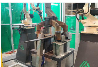
Autoa welding robot in action, repairing a stub.
